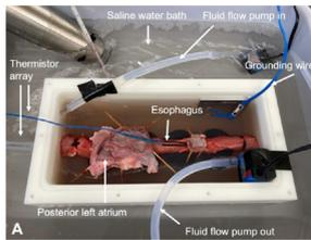
(A): Ex vivo heart-esophageal model used to evaluate temperatures and lag time. (B) Temperature change during ablation with externally irrigated catheter at contact forces of 10-15g for both SA and HPSD methods. (C) From ablation onset, time difference for 1°C rise with SA or 0.5°C rise with HPSD at both AW and esophageal lumen.
